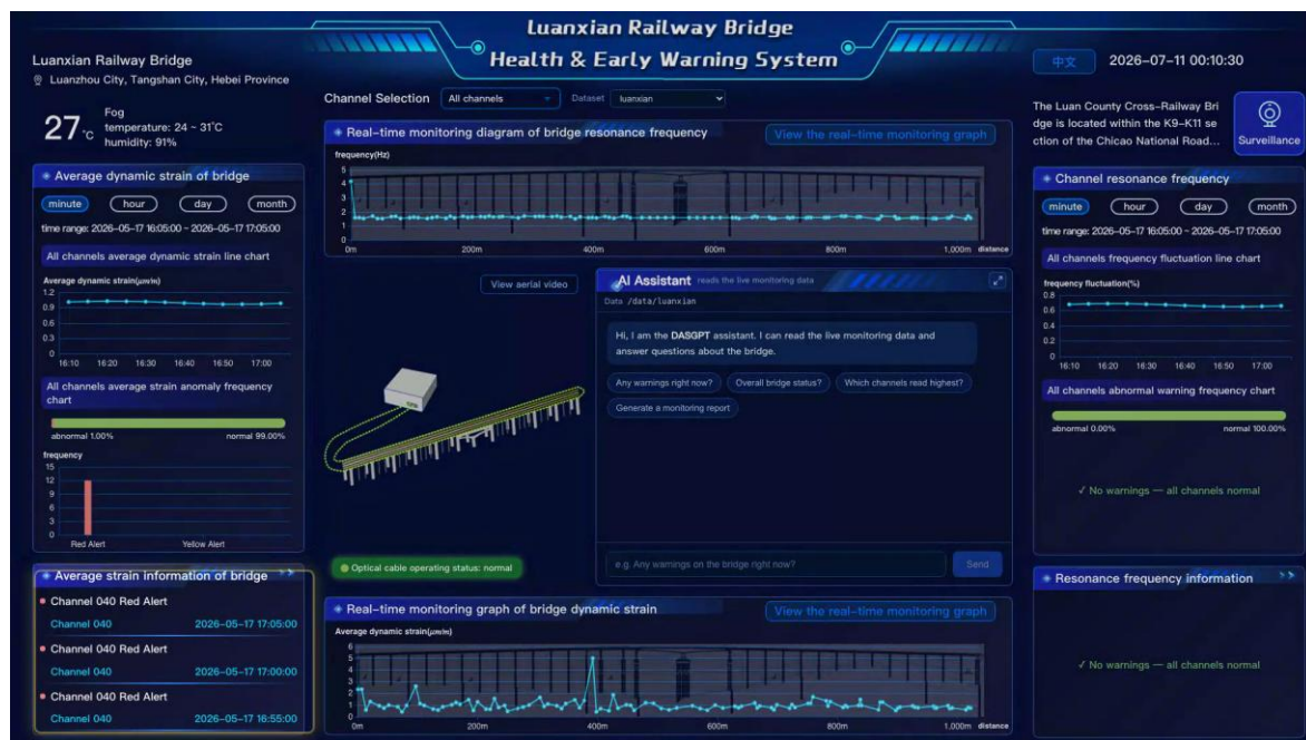
Figure 3-1 · The monitoring dashboard: bridge-shaped health panels, environment strip, and the built-in assistant.
